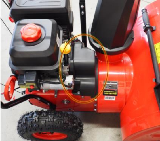
Figure 2. Black plastic cover located between the engine and the discharge chute.
