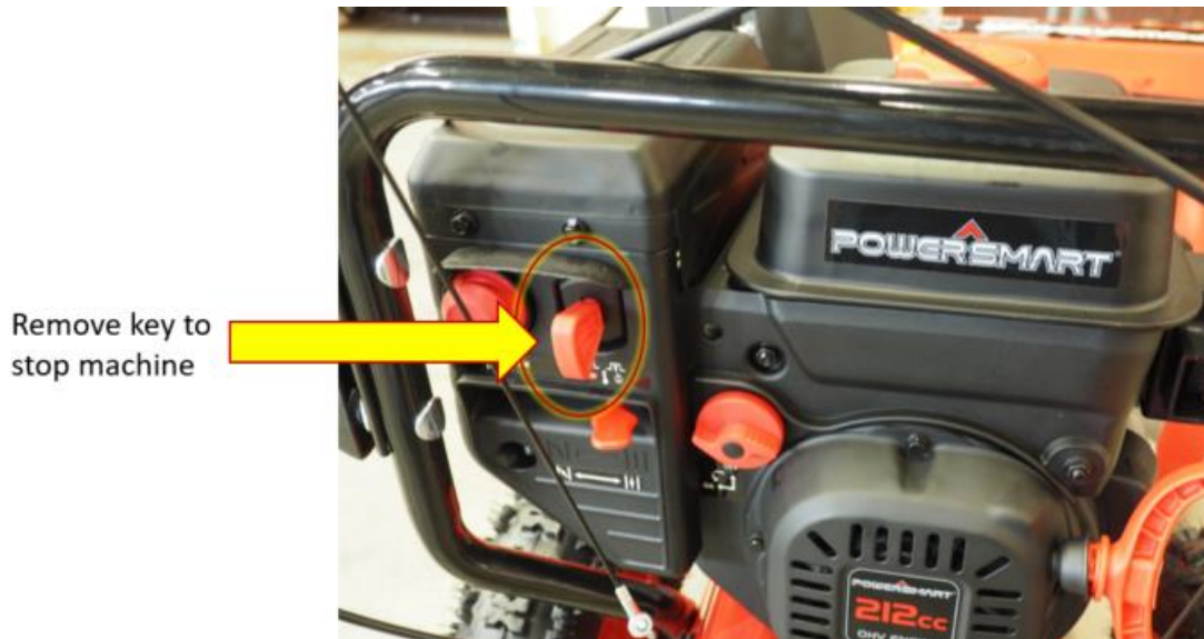
Figure 1. Engine stop safety key; remove in case of unexpected snow thrower motion.
