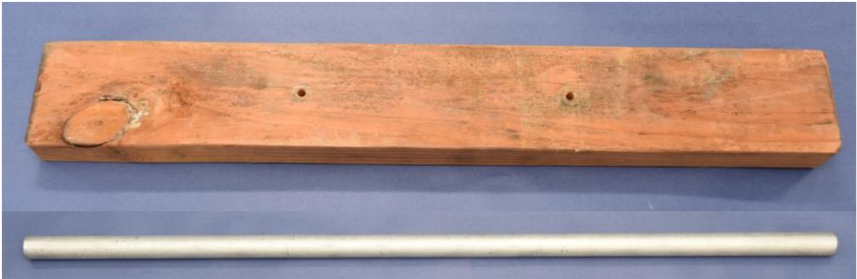
Figure 1. Wood 2 x 4 or stout metal rod that can be used to block the impeller.
